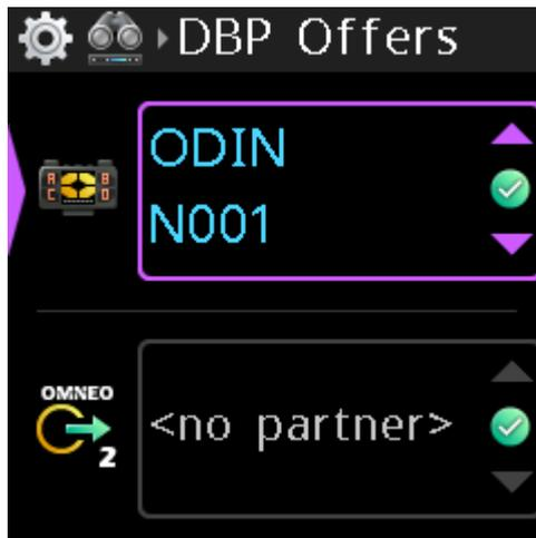
3. Rotate either **shaft encoder** to scroll through the available offers.
