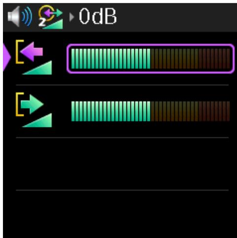
3. Rotate either **shaft encoder** to adjust the level.
