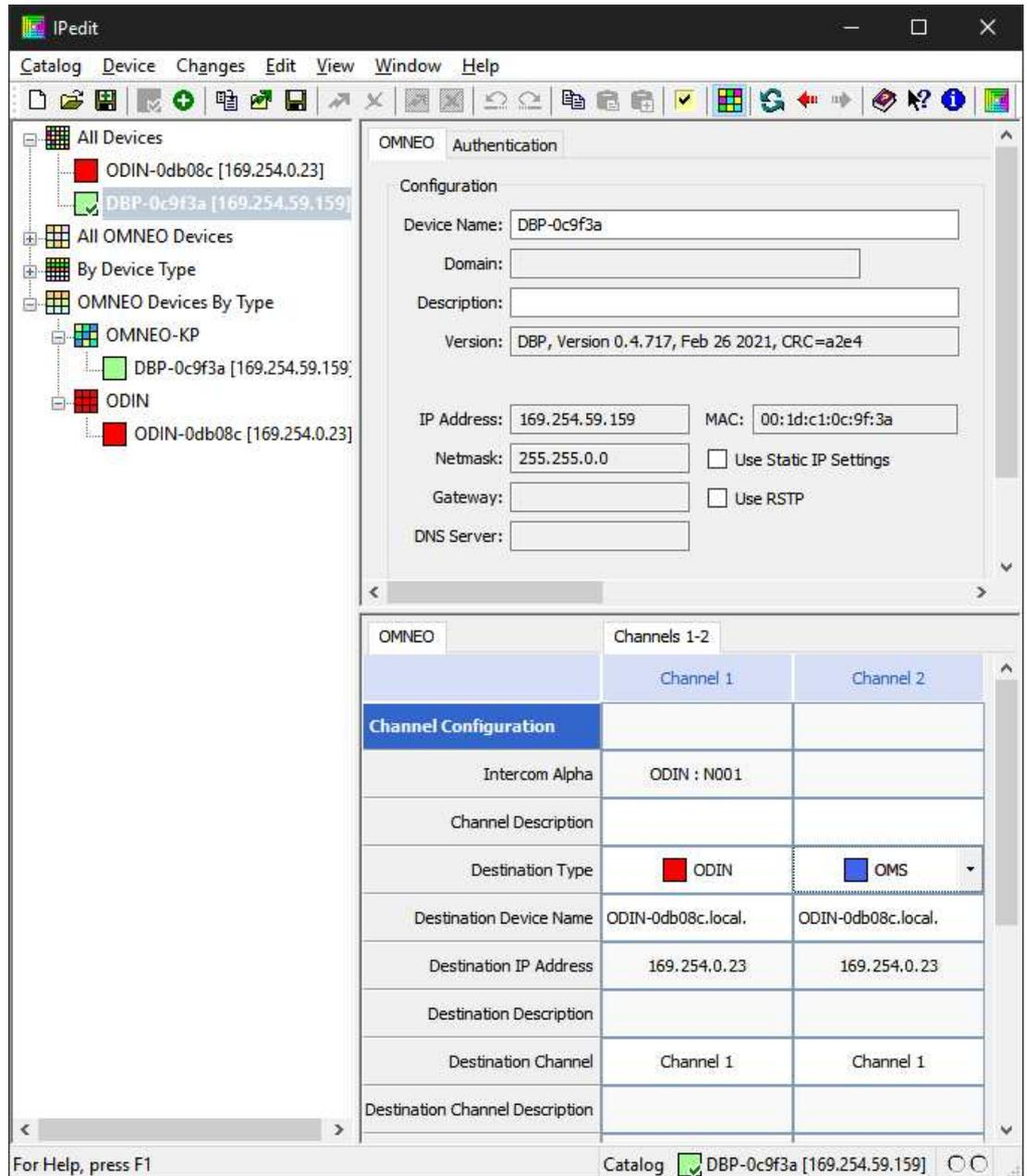
**Using the Channel Configuration Pane**
