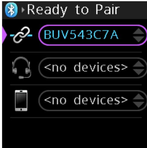
3. Rotate either **shaft encoder** to scroll available devices.
