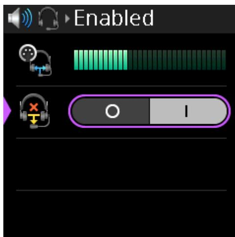
3. Rotate either **shaft encoder** to toggle between choices.
