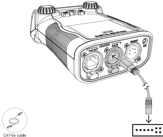
3. Using a second CAT-5e cable, connect **one end to the approved PoE switch**.
