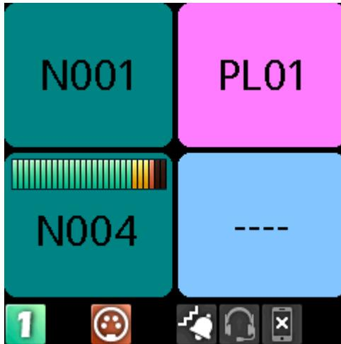
3. Rotate the **A/C shaft encoder** to adjust the volume.
