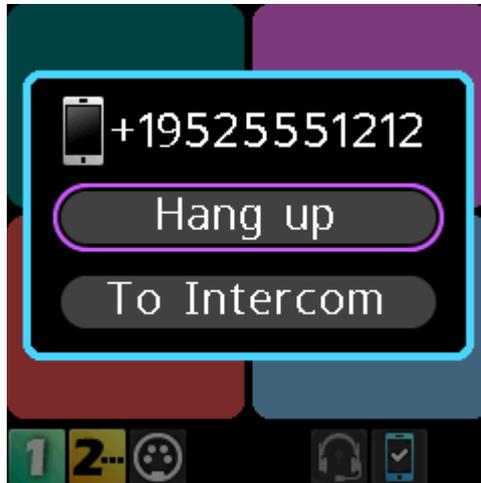
1. Rotate either **shaft encoder** to navigate to To Intercom.
