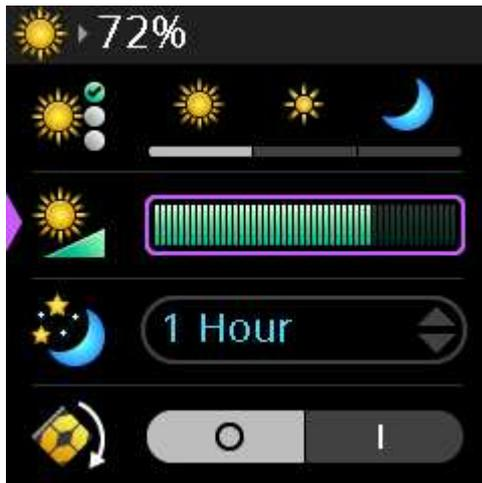
3. Rotate either **shaft encoder** to increase or decrease the display brightness.
