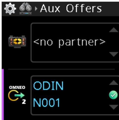
4. Press the **SEL/MENU button** to confirm the change, or press the **CLR/BACK button** to abort changes.
